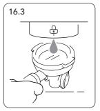
**Backflushing.** Insert the blind filter (C) into the filterholder (G) and pour 1 bag of detergent powder (F or PLA9201) into the filter. Insert the filterholder (G) in the group (6) until the handle is aligned with the padlock symbol placed on the group itself. By pressing the buttons 1 and 4 at the same time, the cleaning will proceed automatically (Pic. 16.2).
